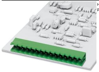
Header, nominal current: 12 A, rated voltage: 250 V, pitch: 5.08 mm, no. of positions: 3, mounting: Soldering
